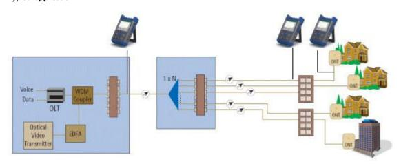
AV6418 OTDR is mainly used to measure FTTx network, it provides multifunctions in one unit. AV6418 offers three measuring modes: manual mode (including real time mode and average mode), auto mode and dead zone mode.
